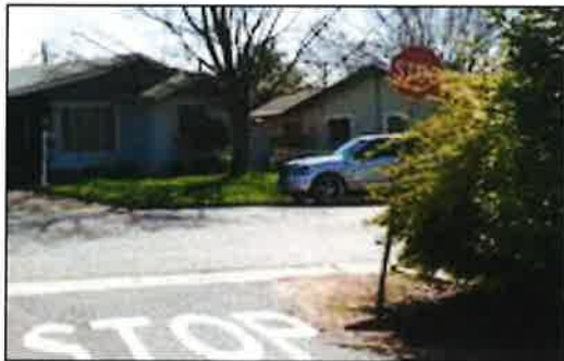
Figure 1: Intersection with Sightline Obstruction
